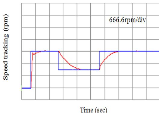
**Figure 10:** Experimental speed tracking of sliding mode controller.
