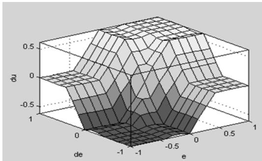
Figure 4: Output of fuzzy logic controller
