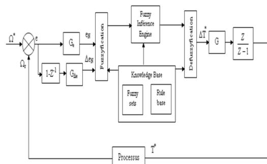
Figure 2: Fuzzy Controller block diagram.
