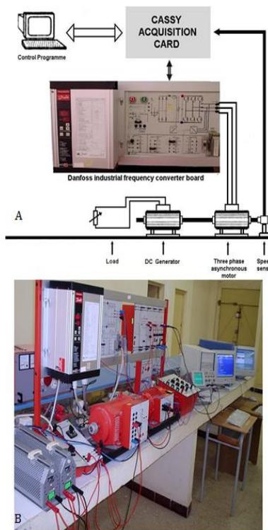
**Figure 7:** Test bed of a scalar controlled induction motor. **A**, Test bed structure; **B**, Test bed photograph.
