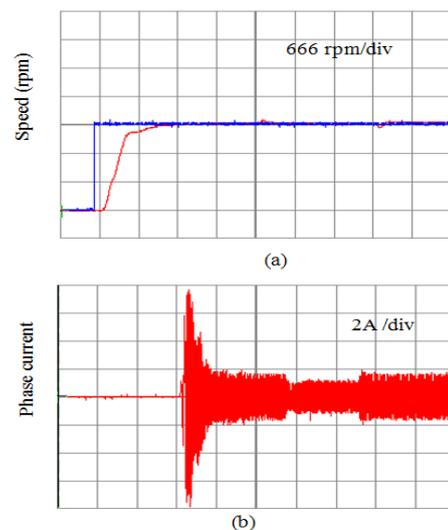
**Figure 9:** Experimental Fuzzy controller Load Torque Disturbance  $\pm (1Nm)$ ; (a) Speed, (b) Phase Current.
