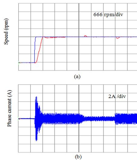
**Figure 8:** Experimental sliding mode controller Load Torque Disturbance  $\pm(1Nm)$ ; (a) Speed, (b) Phase Current.
