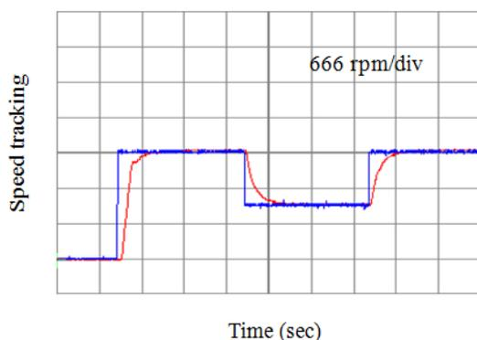
**Figure 11:** Fuzzy Experimental Speed Tracking.
