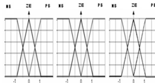
Figure 3: Input and output membership functions.
