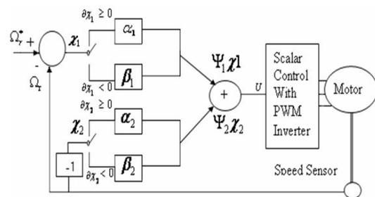
Figure 6: Scalar control showing sliding mode control in detail.
