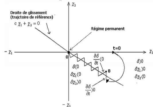
Figure 5: Sliding line control in phase plane X1-X2.
