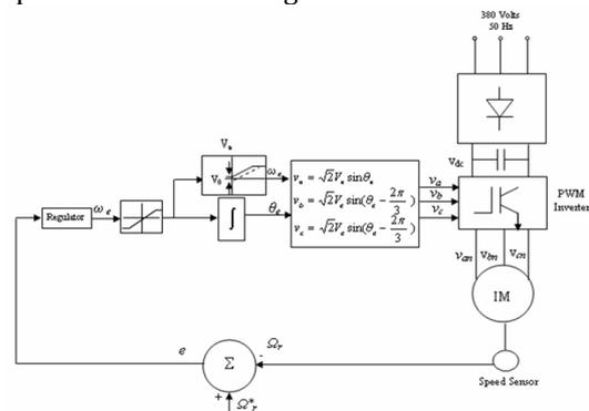
Figure 1: Scalar Control Scheme.
