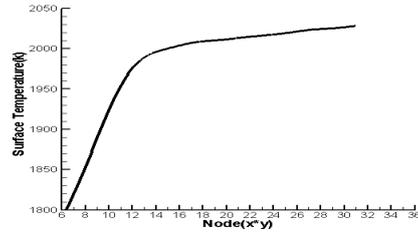
Figure 4: Temperature variation of the surface central point versus number of the nodes.
