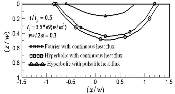
Figure 14: Melting pool image on the x-z plane for a circular laser beam using Fourier and Hyperbolic methods.
