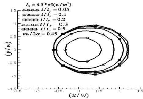
Figure 10: Melting pool image on the x-y plane at a constant velocity and different times for a circular laser beam in continuous heat flux case.
