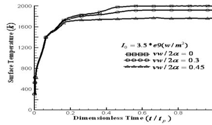
Figure 8: Surface center point temperature with respect to the time at various speeds and intensity of  $I_0=3.5 \times 10^9 \text{ (W/m}^2\text{)}$  in continuous heat flux case.
