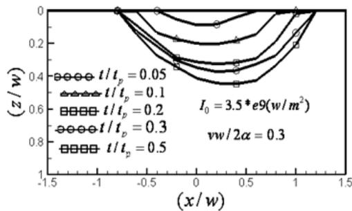
Figure 11: Melting pool image on the x-z plane at a constant velocity and different times for a circular laser beam in continuous heat flux case.
