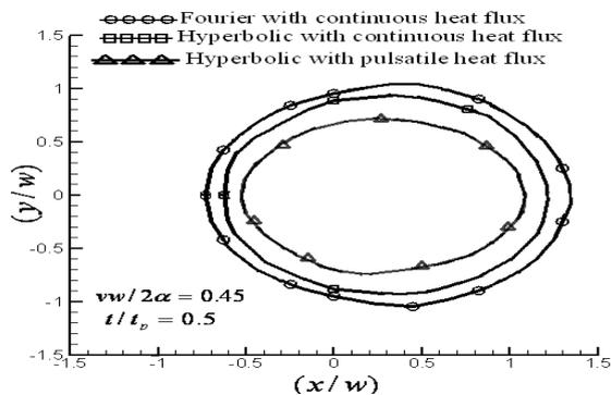
Figure 13: Melting pool image on the x-y plane for a circular laser beam using Fourier and Hyperbolic methods.
