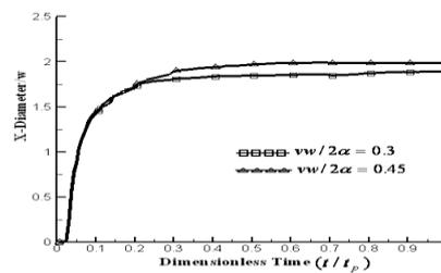
Figure 9: Melting pool diameter on the x-axis with respect to the time for two different speeds in continuous heat flux case.
