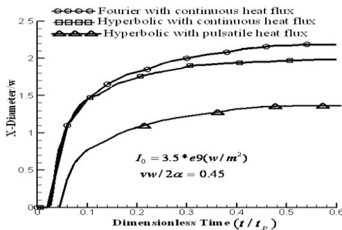
Figure 12: Melting pool diameter on the x-axis versus time using Fourier and Hyperbolic methods.
