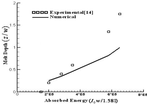
Figure 6: Melting pool depth versus laser beam intensity at the center.
