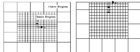
Figure 5: Grid generation in x-y and x-z planes.
