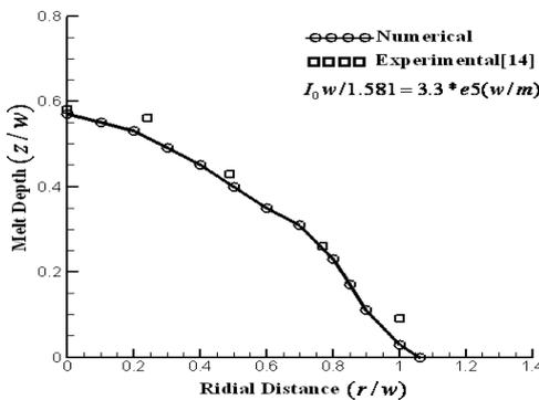
Figure 7: Melting pool depth versus radial distance from the laser beam center.
