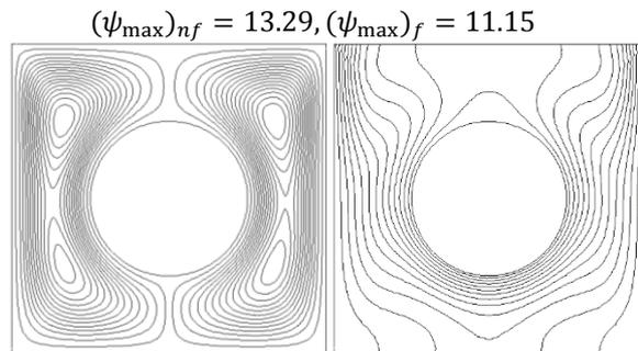
**Figure 3:** Temperature lines (right) and streamlines (left) of the water (base fluid)  $Ra = 10^5, r = 0.25, c(x, y) = (0.5, 0.5)$ .
