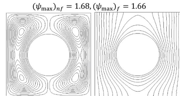
**Figure 2:** Temperature lines (right) and streamlines (left) of the water-copper nanofluid in 6% of volume fraction,  $Ra = 10^4, r = 0.25, c(x, y) = (0.5, 0.5)$ .
