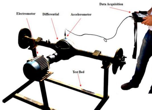
**Figure 1:** Experimental setup included Differential, test bed and etc.
