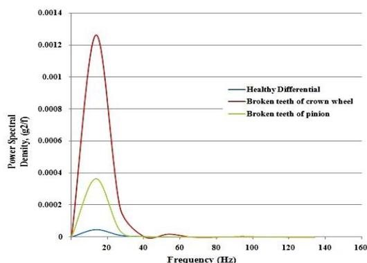
**Figure 6:** Power Spectral Density results of differential.
