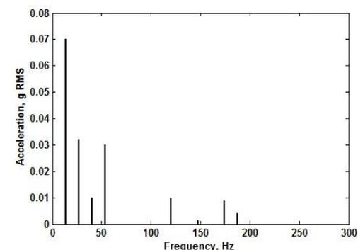
**Figure 5:** Frequency spectrum result of broken teeth of pinion.
