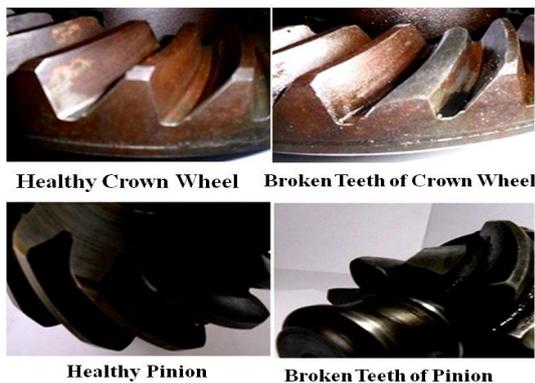
**Figure 2:** Different conditions of crown wheel and pinion.
