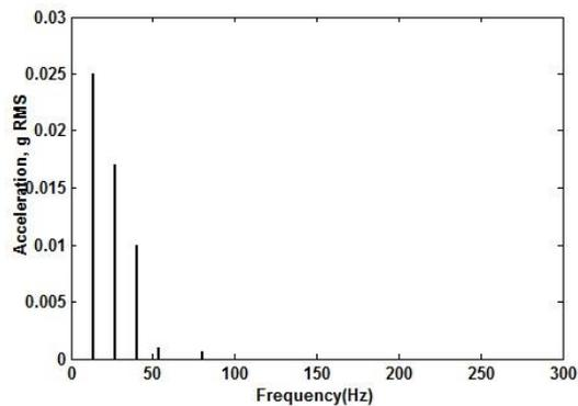
**Figure 3:** Frequency spectrum result of healthy differential.
