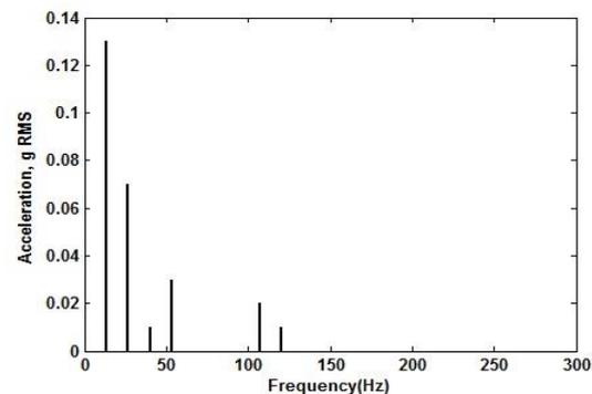
**Figure 4:** Frequency spectrum result of broken teeth of crown wheel.
