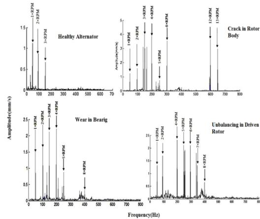
Figure 5: Frequency domain of each class.
