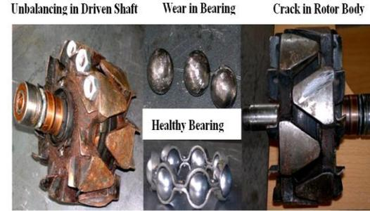
Figure 2: Alternator faults.
