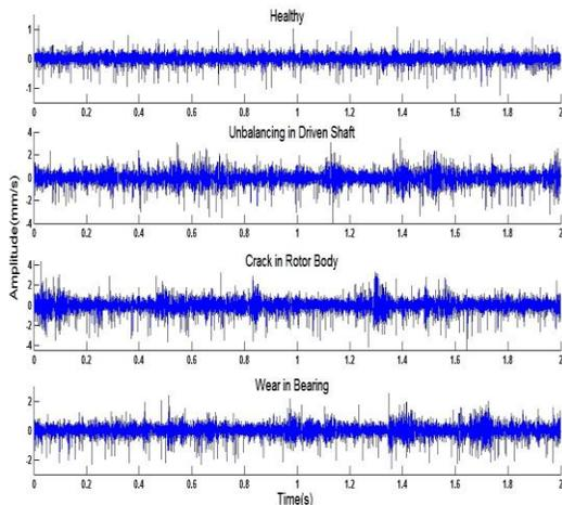
Figure 4: Time signal of each class.
