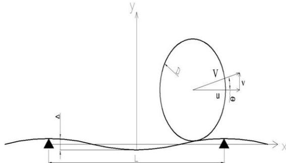
Figure 1: Modeling of rail and wheel
