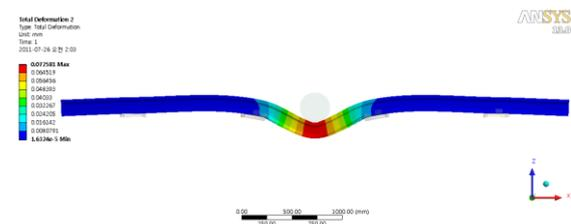
Figure 7: Deflection of rail by span 1200mm
