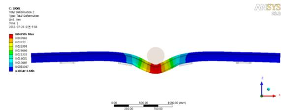
Figure 6: Deflection of rail by span 1000mm
