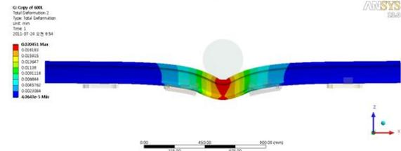
Figure 4: Deflection of rail by span 600mm
