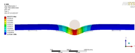
Figure 5: Deflection of rail by span 800mm
