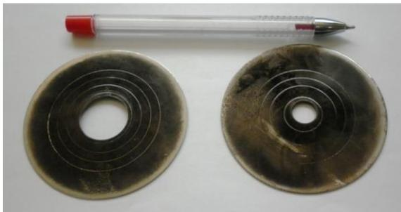
**Figure 12:** Experimental test samples for obtaining the limits of effective scan radius
