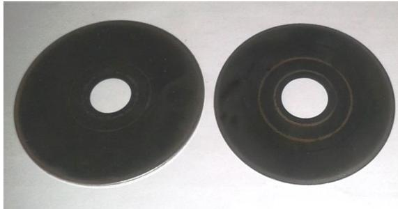
**Figure 13:** Experimental test samples for obtaining the minimum of effective hole diameter (with ID 15 mm and 18 mm)
