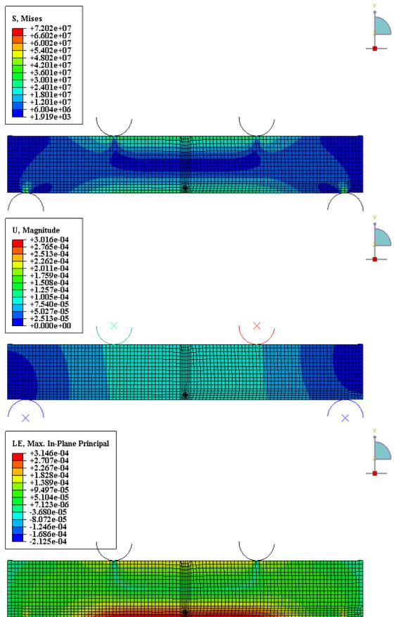
Figure 2: Stress, deflection and strain in type2 of model
