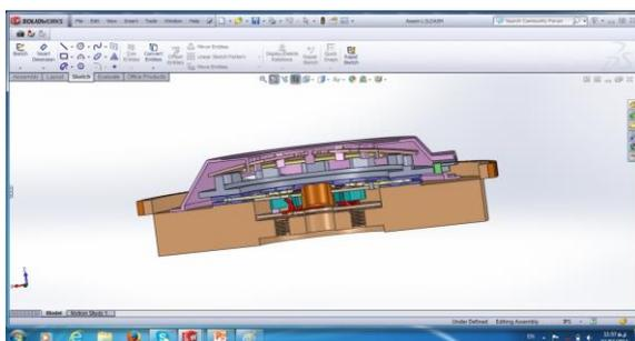
**Figure 7:** A Section of Clutch Set
