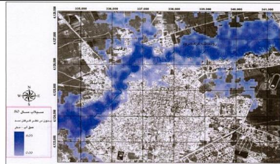
Figure 4: Maximum flood depth in the plain
