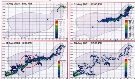
Figure 3: Flood zoning for the maximum occurred flood.
