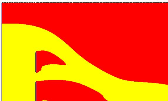
**Figure 8:** Simulated flow passing over and under the combined weir-gate
