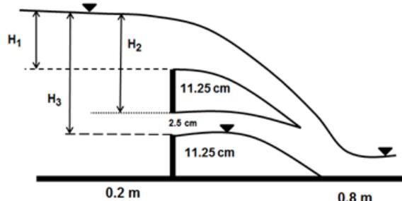
Figure 6: Details of flow passing the combined weir-gate with 10 % gate opening.
