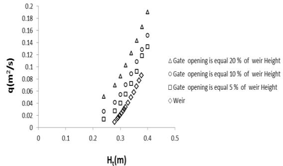
**Figure 9:** Variation of discharge versus  $H_t$  in studied models
