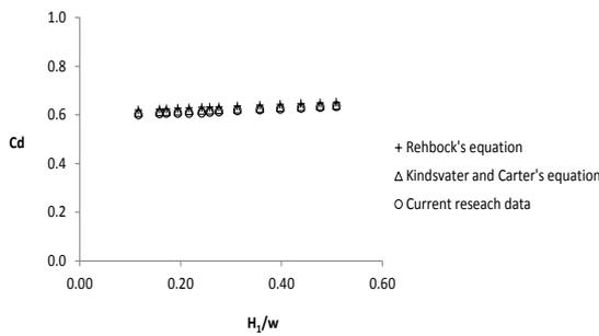
**Figure 7:** Variation of Discharge coefficient values versus  $\frac{H_1}{w}$  for single weir
