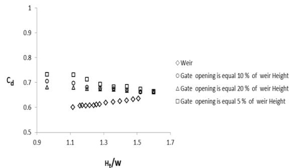
**Figure 10:** Variation of discharge coefficient versus  $\frac{H_t}{w}$  in studied models
