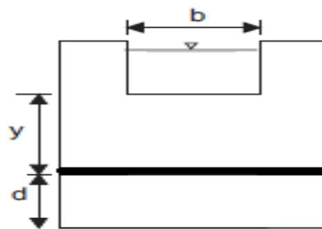
**Figure 3:** Cross section of combined weir-gate gate with unequal contractions
