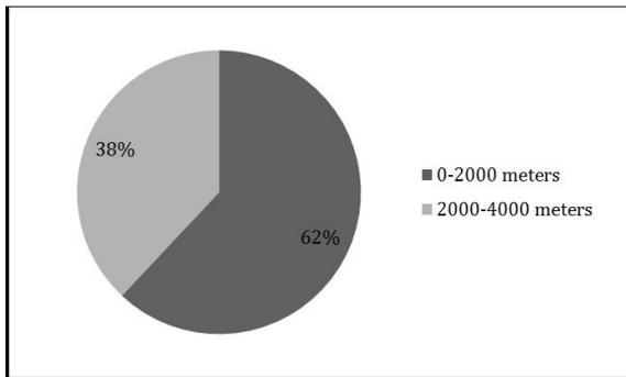
Figure 5: stuck pipe distribution regarding depth.
