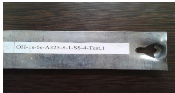
Figure 12: Side view of connection failure
