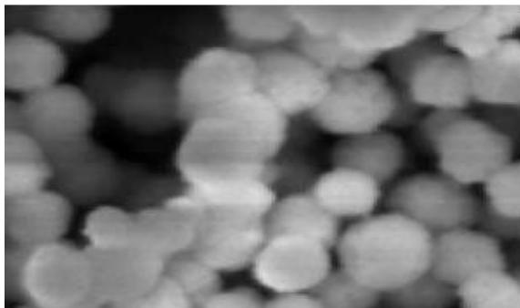
Figure 3: SEM picture and TEM picture of the copper nanoparticles
