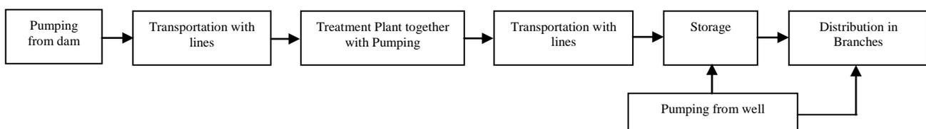
Figure 2. Process of water distribution
