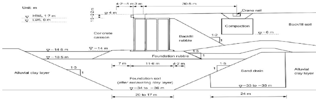
Figure 1. cross-section of Caisson Wharf of Island Rokko in Kobeh port
