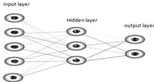
Figure 1. Structure of multi-layer perceptron neural network
