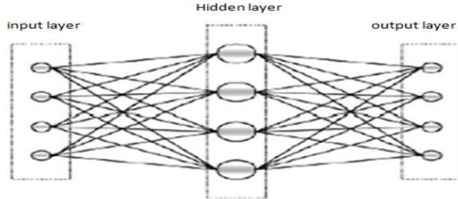
Figure 2. Structure of radial basis function of neural network structure
