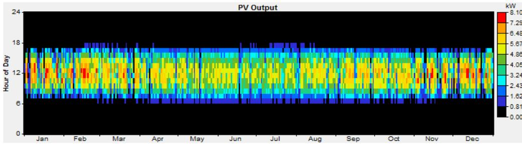
Figure .7 the amount of energy produced from photovoltaic cells over a year
