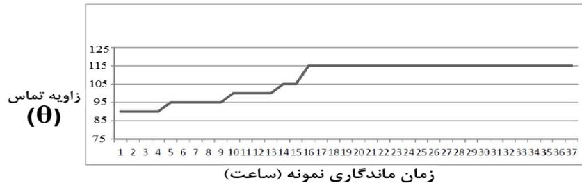
Figure 15. contact angle results in terms of samples duration in drilling mud
