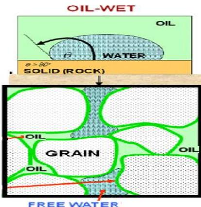
Figure 9. Oelophilic properties of reservoir rock by filling small pores
