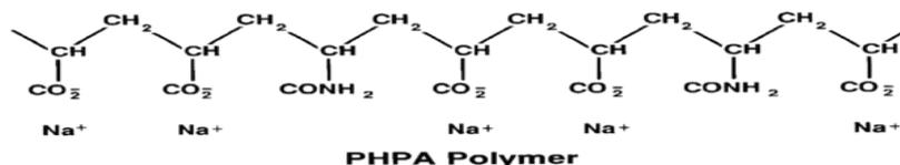
Figure 1. PHP Molecular structure
