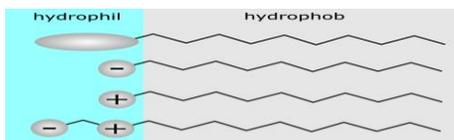
Figure 11. the surfactant performance. Polar head in polar environment and nonpolar head in Oelophilic environment
