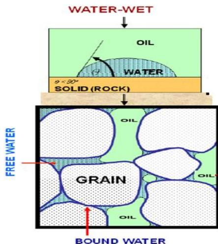
Figure 7. hydrophilic properties of reservoir rock by filling the small pores
