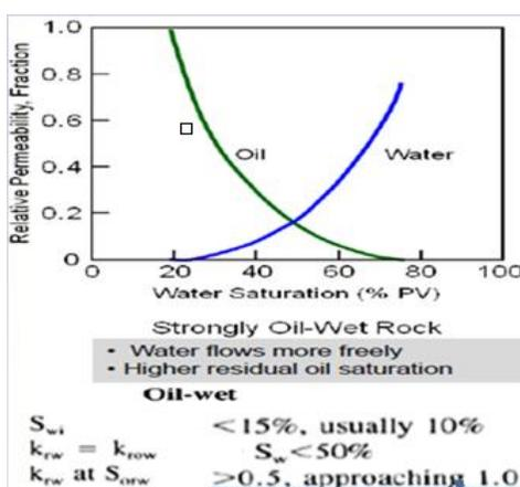
Figure 10. increasing the relative permeability of water ( $K_{rw}$ )
