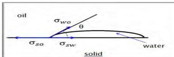
Figure 5. the solid surface in the presence of water and oil
