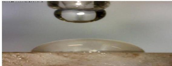
Figure 16. a water drop in reservoir in the vicinity of the mineral calcite
