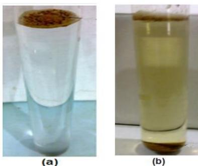
Figure 18. Flotation test a) Oelophilic b) hydrophilic (with surfactant)
