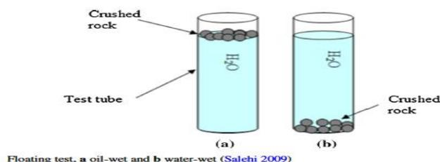
Figure 17. Flotation test Salehi model a) Oelophilic b) hydrophilic
