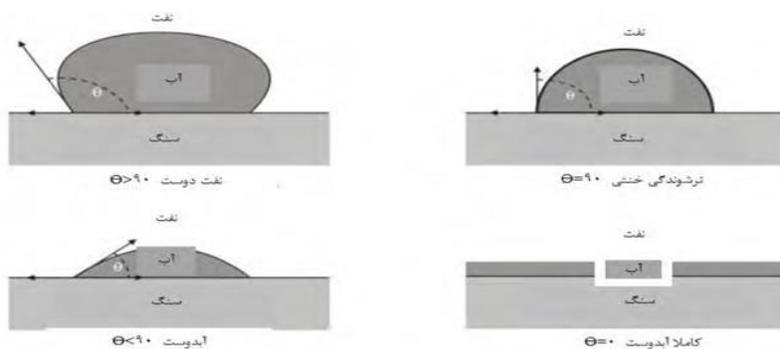
Figure 6. the contact angle in different wettability situations
