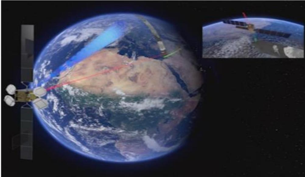
Figure 4. Connection between imaging satellite on LEO orbit with satellite on GEO orbit by laser system
