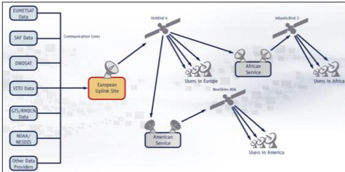
Figure 3. Nodes European section GEONETCast network
