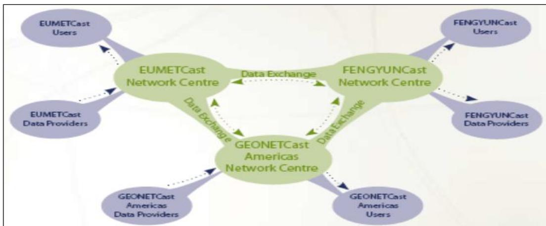
Figure 1. GEONETCast system topology
